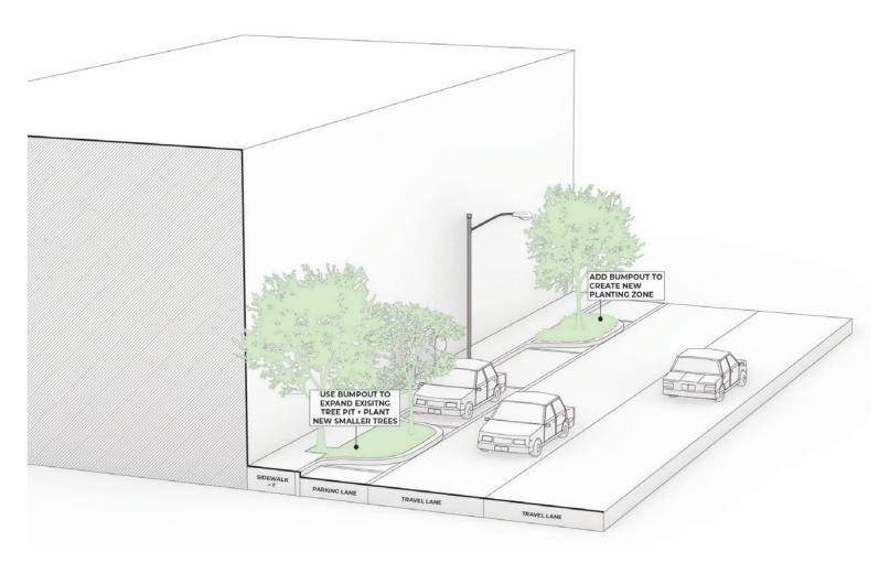
**Bump-outs.** Where sidewalk space is insufficient to plant and reduction of travel and parking lane width is not possible, bumpouts can create space for street trees. Intermittent removal of parking spaces to allow for tree planting can provide for new tree planting and for additional soil space for existing trees with limited soil volume. Small trees at adequate distance from existing trees may also be added to create a biodiverse and layered canopy.
