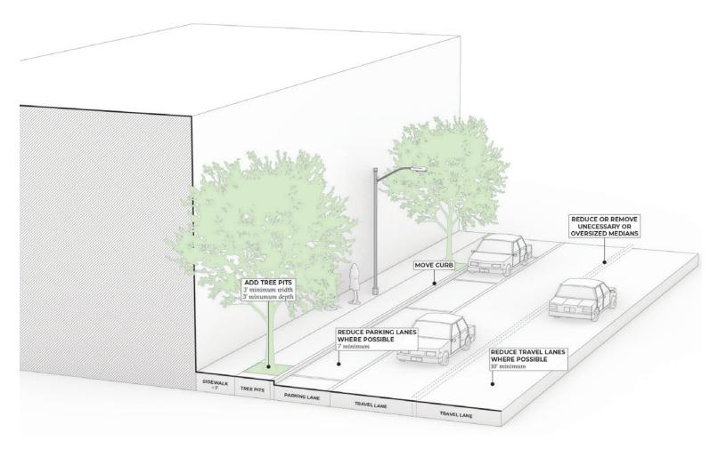
**Reduce Street Widths.** Multiple means to make space for street trees can be employed including; reducing the width of travel or parking lanes and removing or reducing the width of existing medians. Depending on exact site conditions these measures, alone or combined, can create sufficient space for planting street trees.
